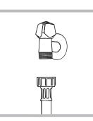
1. Connect the supply pipe by screwing it to a cold water tab using a <sup>3</sup>/<sub>4</sub> gas threaded connection *(see figure).* Before performing the connection, allow the water to run freely until it is perfectly clear.
